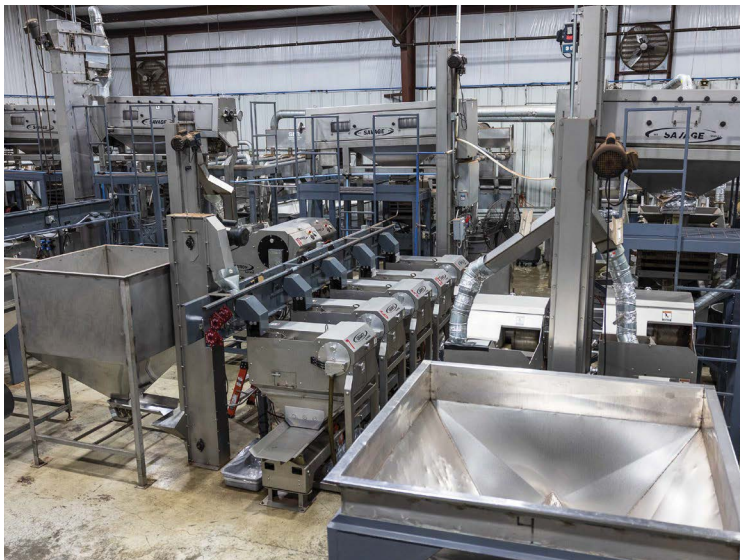
The Millers' processing plant sizes, cracks and sorts pecans.
